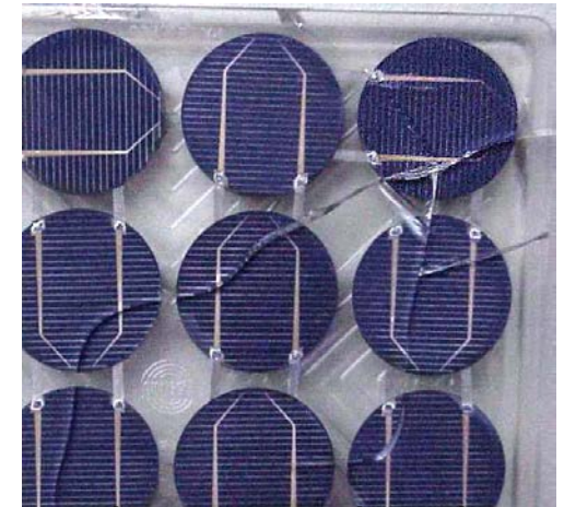
Cracked glass due to overheating
